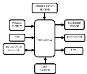
Figure 1. Block Diagram
